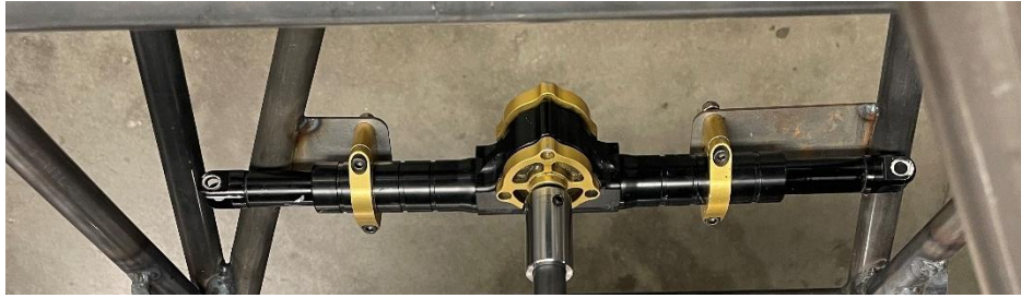
Figure 5: KAZ Technologies Steering rack mounted into frame, Top view
