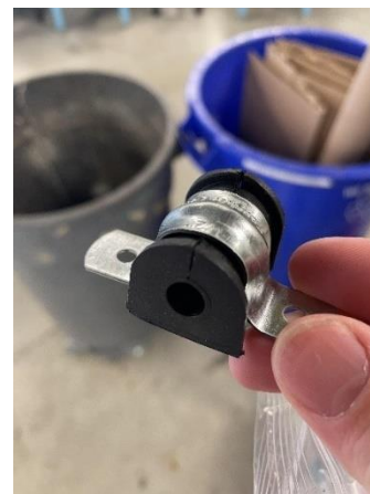
Figure 10: Rubber bushing, with a 3/8 in hole that would hold the Anti Roll Bar in place
