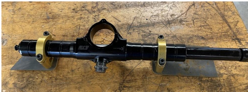
Figure 8: KAZ Steering rack with Tabs, 0.125" Thck, Plain Carbon Steel
