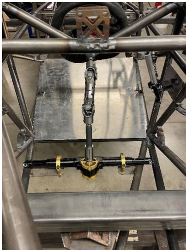
Figure 16: Off center steering rack after the rack was initially installed in the car
