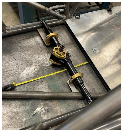
Figure 9: Steering rack location before being tacked into place, using a tape measure to ensure the location is correct
