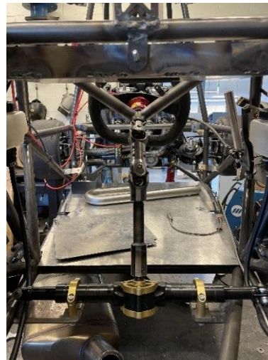
Figure 17: Looking straight down the center, after resolving the off center steering column
