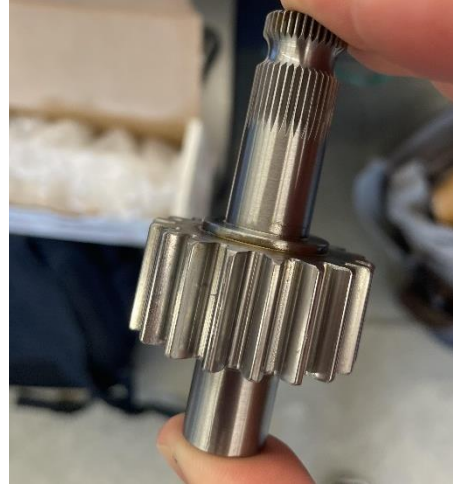
Figure 2: New Pinion Gear, Note the splines not being chewed up, steel
