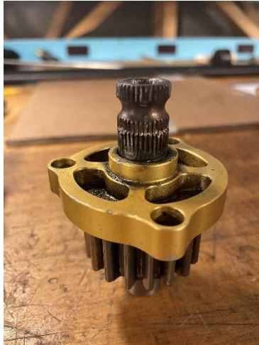
Figure 1: Old Pinion from KAZ Tech. Steering Rack vs New Rack, Note splines
