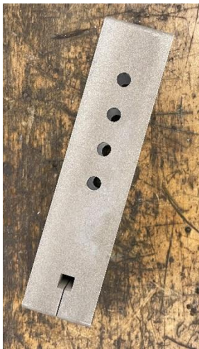
Figure 25: Anti Roll Bar End link: 6061-T6 Al.
