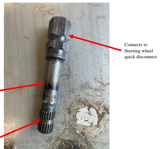
Figure 14: Upper steering column assembly, Steel
