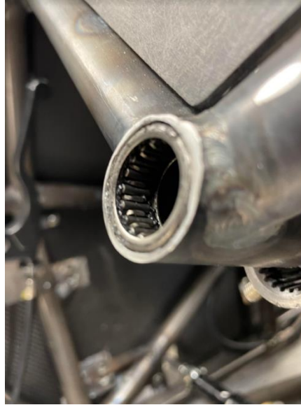
Figure 12: Steering Column Mount, with 1" OD Bearing, 0.750" ID
