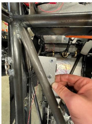
Figure 11: 0.125" Thick, Steel Tab used to hold up the Anti Roll bar. This tab was modified to fit the awkward frame member
